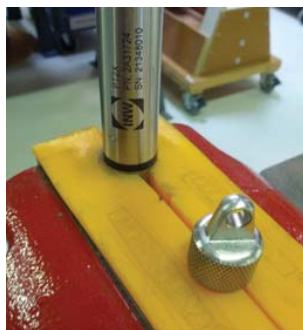
Cableless Sensor - gripping on knurled area
