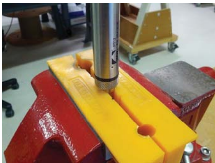
Cabled Sensor - gripping on swage
