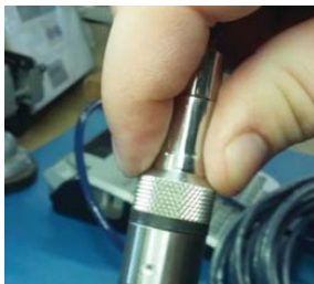
Properly completed — black ring uncompressed
