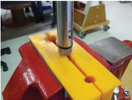
Cabled Sensor - gripping on swage
