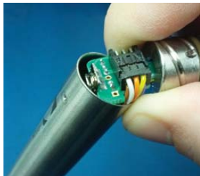
Wires tucked into slot and spring tucked into housing.
