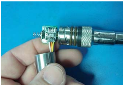
Connector connected properly
