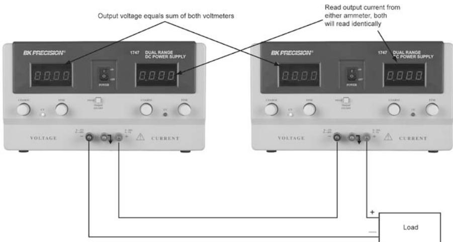
Figure 8 - Connecting Two Power Supplies in Series
