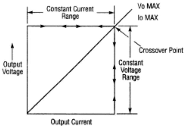
Figure 7 - Constant Voltage/Constant Current Characteristic
