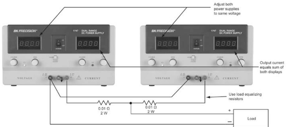
**Figure 9 - Connecting Two Power Supplies in Parallel**
